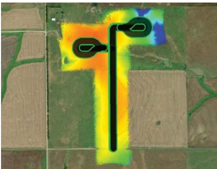
The required Area of Interest overlaid on top of a LiDAR point cloud which is colorized to show elevation. This image illustrates complete coverage for quality assurance
