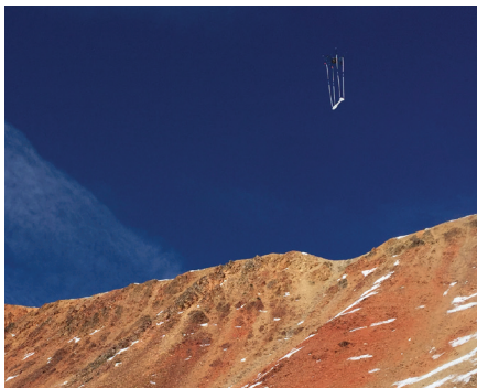
Magnetometer flown on the DJI Matrice 600 Pro at over 12,000' in the project area.
